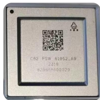
•PCIe Switch芯片
